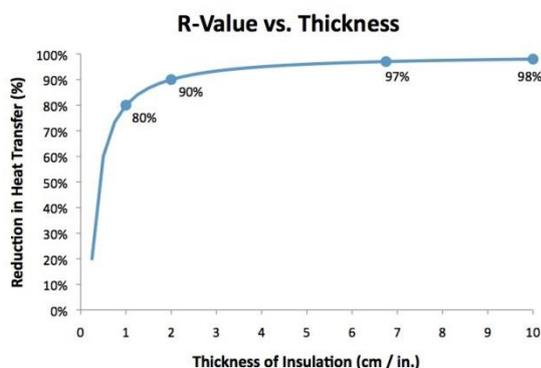
There is a substantial difference between insulation for temperature control and insulation for heat loss control. For instance, the graph (below) shows the heat loss control of the spray-in-place urethane foam insulation. Any insulation will have a similar graph but with thicker amounts of insulation. This graph points out that more insulation is not necessarily cost effective. There is a point where more insulation is pointless from a total heat loss perspective.
